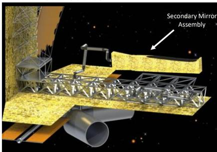
Figure 12. Artistic depiction of robotic assembly of the secondary mirror module
