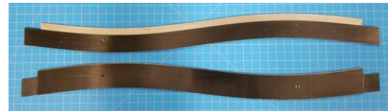
Half length (0.5m) edge prototype (top – telescope side, bottom – Star side)
