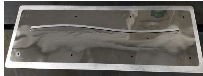
5. Develop resist, prescribing desired in-plane profile
