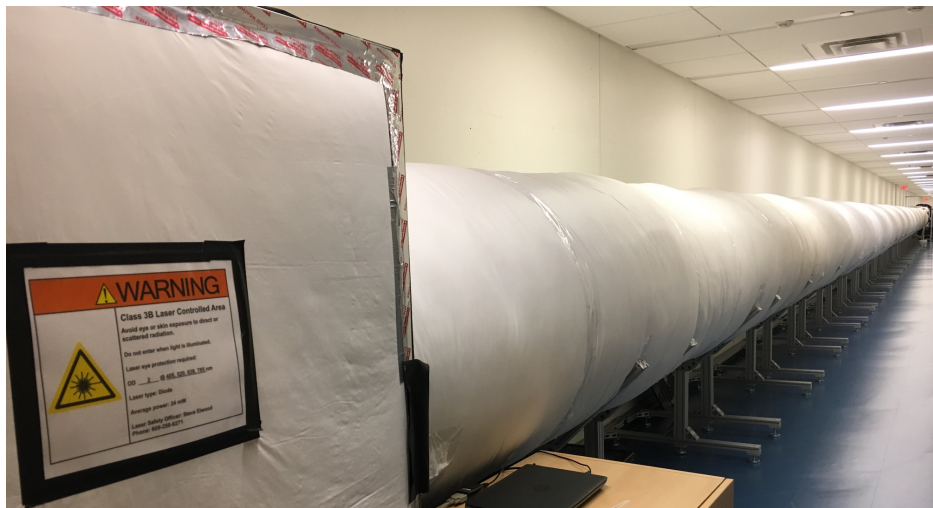
Figure 2: Standing at the camera station and looking down the length of the testbed toward the mask and laser stations. The white insulation minimizes the effects of external temperature fluctuations.
