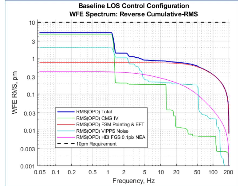
Reverse-cumulative RMS separated in two spatial frequency bins (left) and by error source (right) WFE for worst-case structural dynamic model; different noise sources are activated to compare the relative contribution of each; compliance with a nominal 10 pm RMS WFE requirement is predicted
