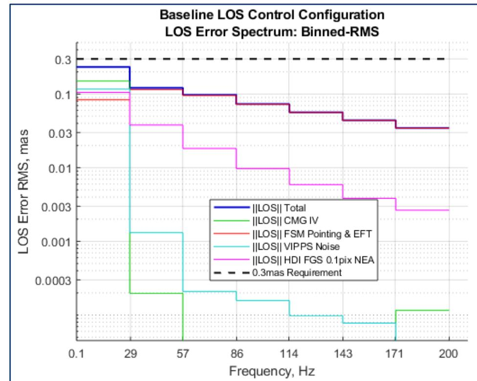
Reverse-cumulative RMS (left) and binned RMS (right) LOS error for worst-case structural dynamic model; different noise sources are activated to compare the relative contribution of each; performance slightly exceeds 0.3 mas requirement, but compliance can be recovered by reducing FSM servo control bandwidth
