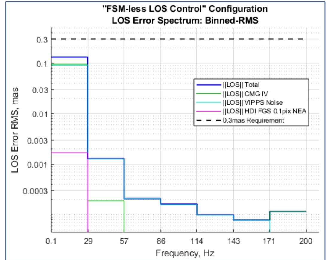
Reverse-cumulative RMS (left) and binned RMS (right) LOS error assuming no FSM in control system; compliance to LOS error is predicted with margin
