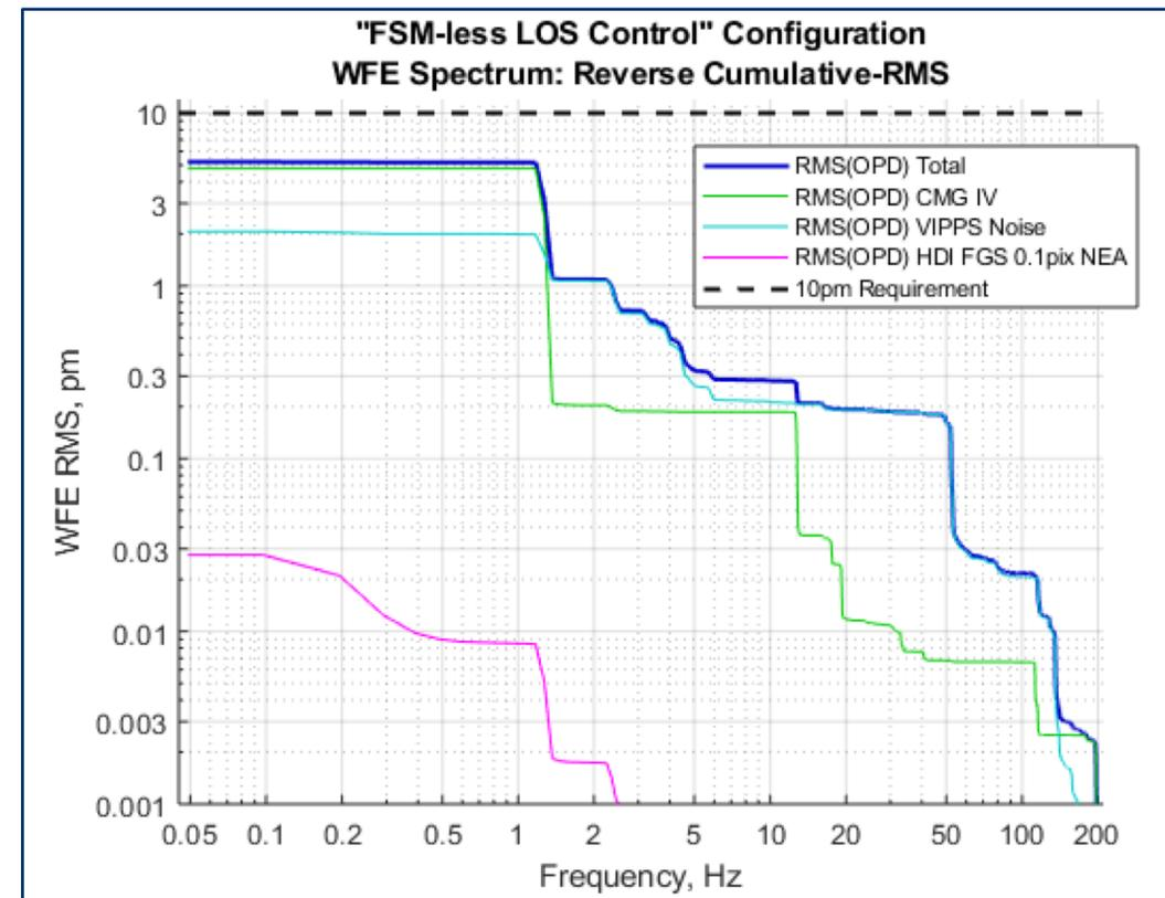
Reverse-cumulative RMS separated in two spatial frequency bins (left) and by error source (right) WFE assuming no FSM in control system; WFE performance is not appreciably altered by presence or absence of FSM
