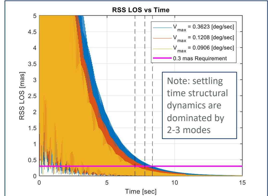
The plots above show RMS WFE (left) and Root-Sum-Square (RSS) of LOS error after slew completion (horizontal axis is time since slew end); results show that over a broad range of maximum slew velocity (greater than required min rate of 0.09 deg/sec) settling time is less than about 10 minutes
