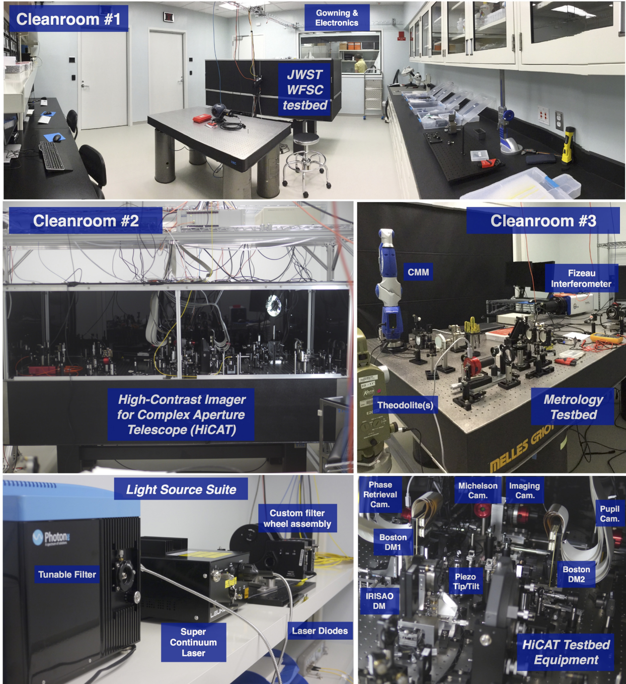
FIGURE 1. Russell B. Makidon Optics Laboratory Facilities and Equipment. Cleanroom facilities provide cleanliness (operated at ISO-6 / class 1000 level), temperature and humidity controlled environment. Cleanroom #1 hosts the JWST Optical Simulation Testbed (JOST). Cleanroom #2 and #3 host the HiCAT testbed and its associated Metrology Testbed described in this proposal. General major equipment includes several light sources (laser diodes, HeNe laser, supercontinuum laser and tunable filter). The metrology testbed includes a Fizeau interferometer, and the lab can borrow a coordinate measurement machine and Theodolites when needed. The HiCAT testbed includes three deformable mirrors, several cameras, and piezo tip/tilt control.
