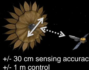
Testbed validated model of sensing accuracy; simulated control performance under flight-like conditions.
