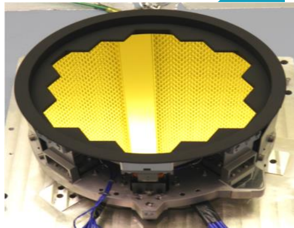
JWST Fine Steering Mirror with 24 Hz bandwidth and 16 mas resolution. UV-VIS FSM will need \sim < 0.1\text{mas} resolution, higher bandwidth and wider range.
