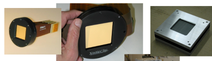
Evolution of monolithic PMN deformable mirrors: left to right: 32x32 array, used for all HCIT milestones to date; 64x64 array to be installed on HCIT spring 2009; 48x48 array (also shown on JPL shake table) will be used to demonstrate TRL6 right readiness this year.
