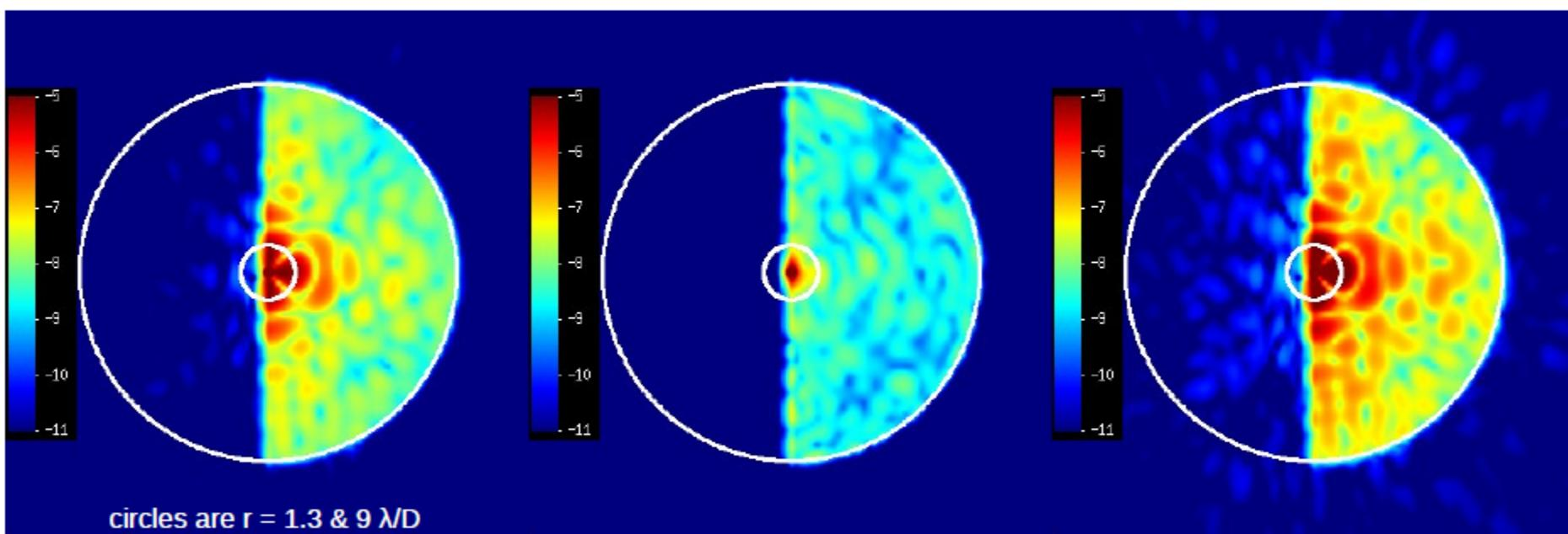
1 DM used to form a half dark hole.
