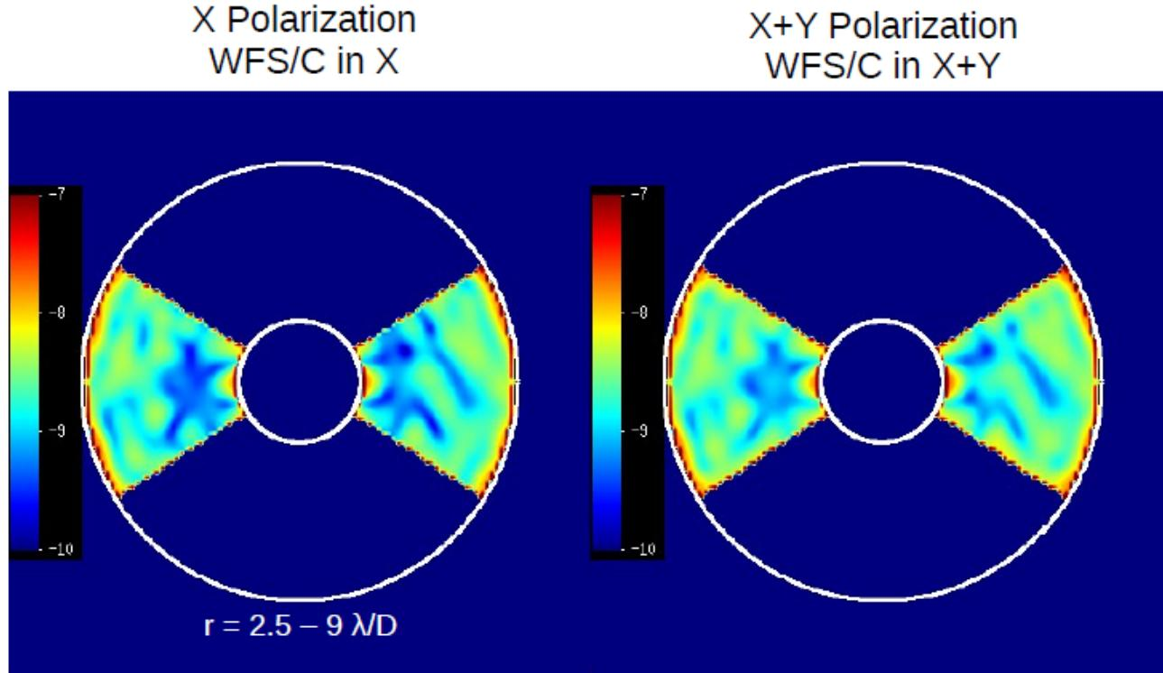
The shaped pupil + Lyot stop is only mildly sensitive to polarization errors. The primary aberration differences between the X and Y polarizations are astigmatism and tilt, both of which this design is relatively insensitive to. The polarization-induced aberrations are a few times less at 550 nm than 800 nm.
