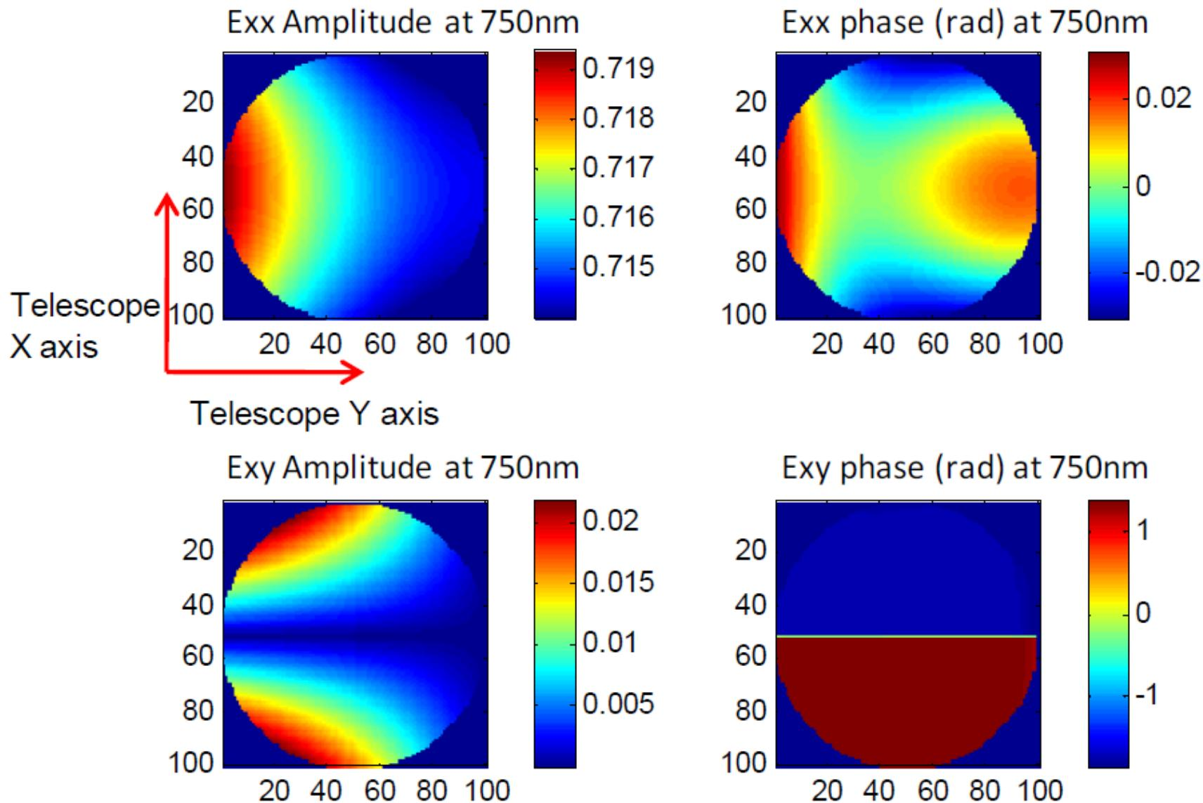
Figure 8. Exx and Exy field pupil maps with the telescope mirrors coated with 25nm MgF<sub>2</sub> protected Al
