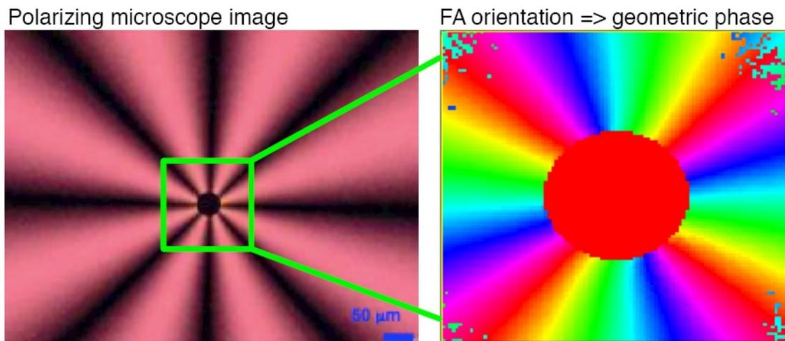
**Figure 2.** *Left: A fourth-order liquid crystal polymer vortex phase mask between crossed polarizers. Right: zoom on the central part using a polarimetric microscope, as measured at the Univ. of Arizona, showing the fast axis orientation rotating about the center. Here, this rotation yields a geometric phase change equals to  $4\theta$ , where  $\theta$  is the focal plane azimuthal coordinate, subsequently spanning 4 waves or  $8\pi$ . (Mawet et al. 2011b).*
