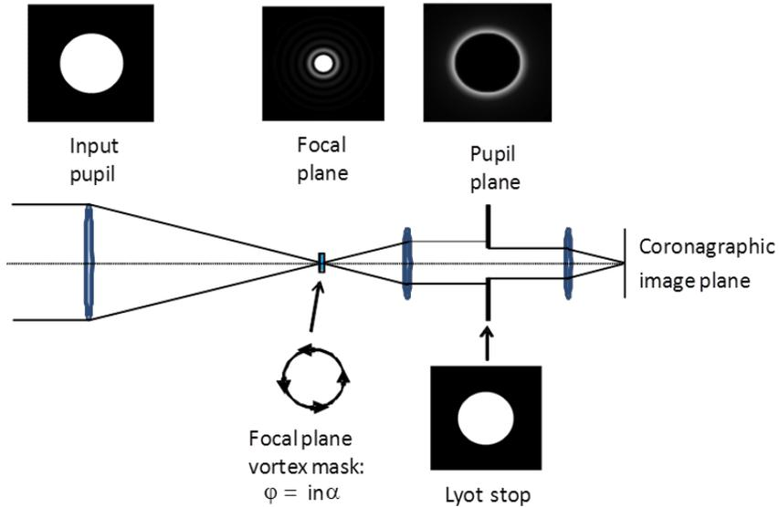
**Figure 1.** Layout of the optical vortex coronagraph: an optical vortex phase mask in the focal plane yields a downstream pupil image in which all of the on-axis starlight appears outside of the original pupil's image, where it is blocked by an aperture (Lyot) stop.
