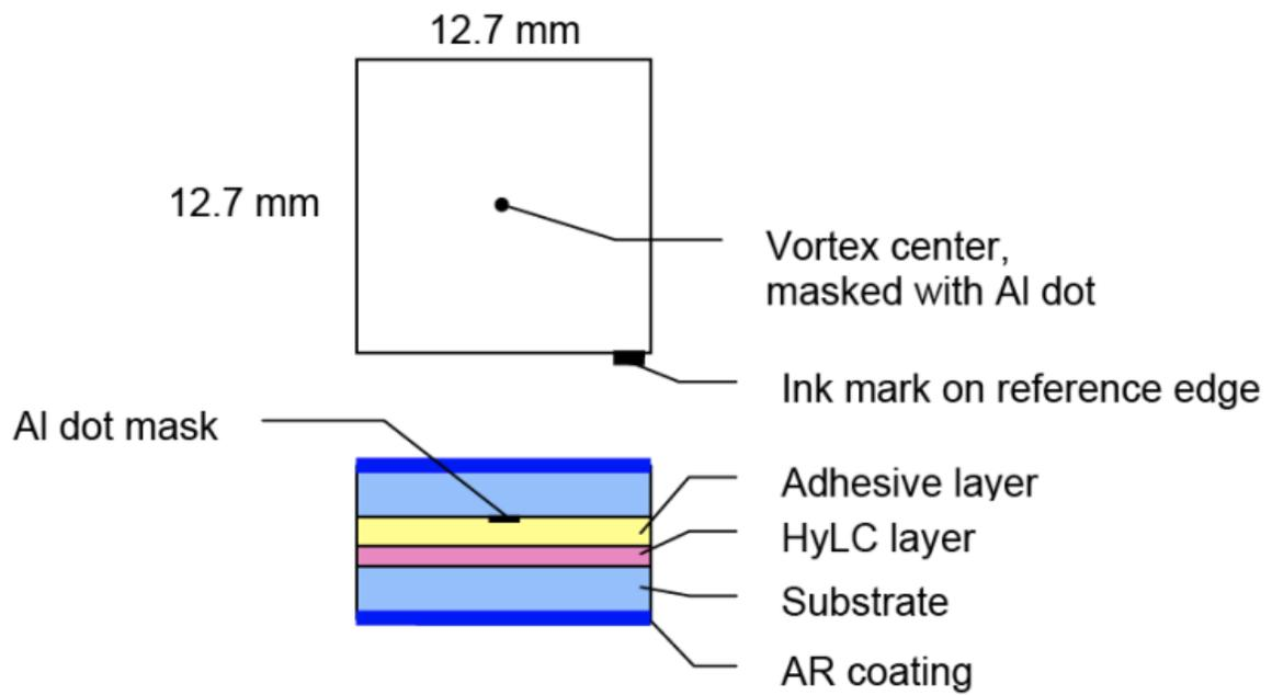
**Figure 3.** *Cross-section of the sandwich design of the JDSU liquid crystal polymer vortex mask. The hybrid liquid crystal polymer (HyLC) layer is deposited on one substrate and a small opaque dot mask is placed upon another substrate, and the two are then glued together, with the dot centered over the vortex.*
