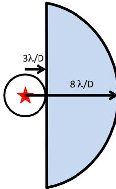
**Figure 5.** Target high-contrast dark field. As described in the text, inner and outer regions are defined for the one-sided dark field. The location of the suppressed central star is indicated in red. The target dark hole for this initial demonstration is from 3 to  $8 \lambda / D$ , as defined in this figure.
