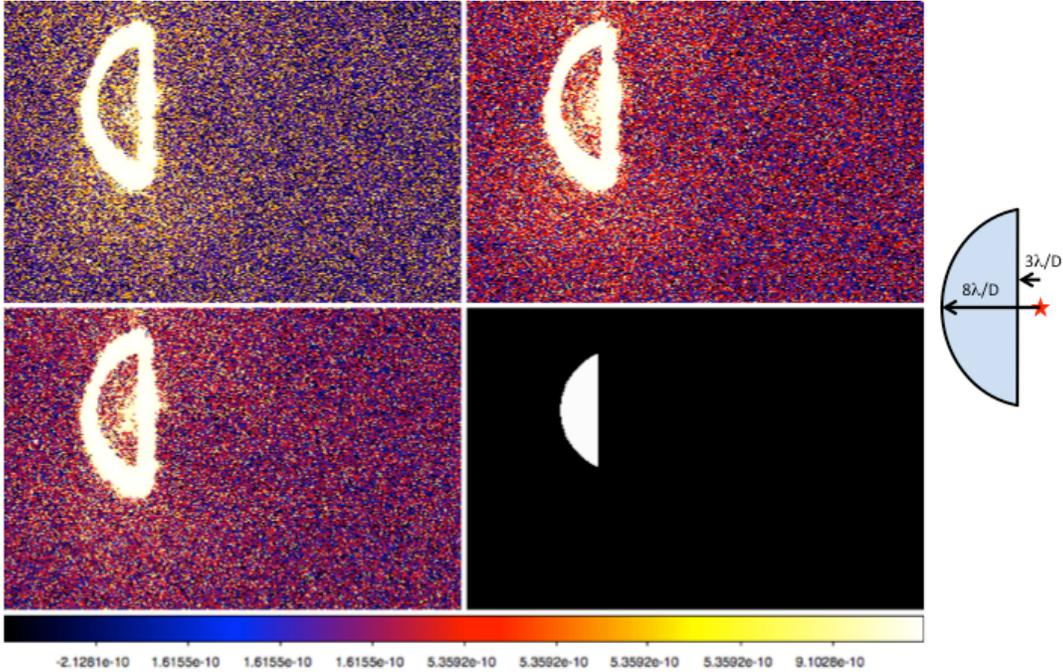
**Figure 8a.** Right-hand edge: Schematic of the size and location of the targeted  $3\text{--}8 \lambda/D$  dark hole relative to the location of the point source (red star) in the image plane. Colored panels: three images showing the final dark holes obtained at the end of the three independent milestone nulling runs. Bottom right: the size and location of the  $3\text{--}8 \lambda/D$  dark hole on the same spatial scale.
