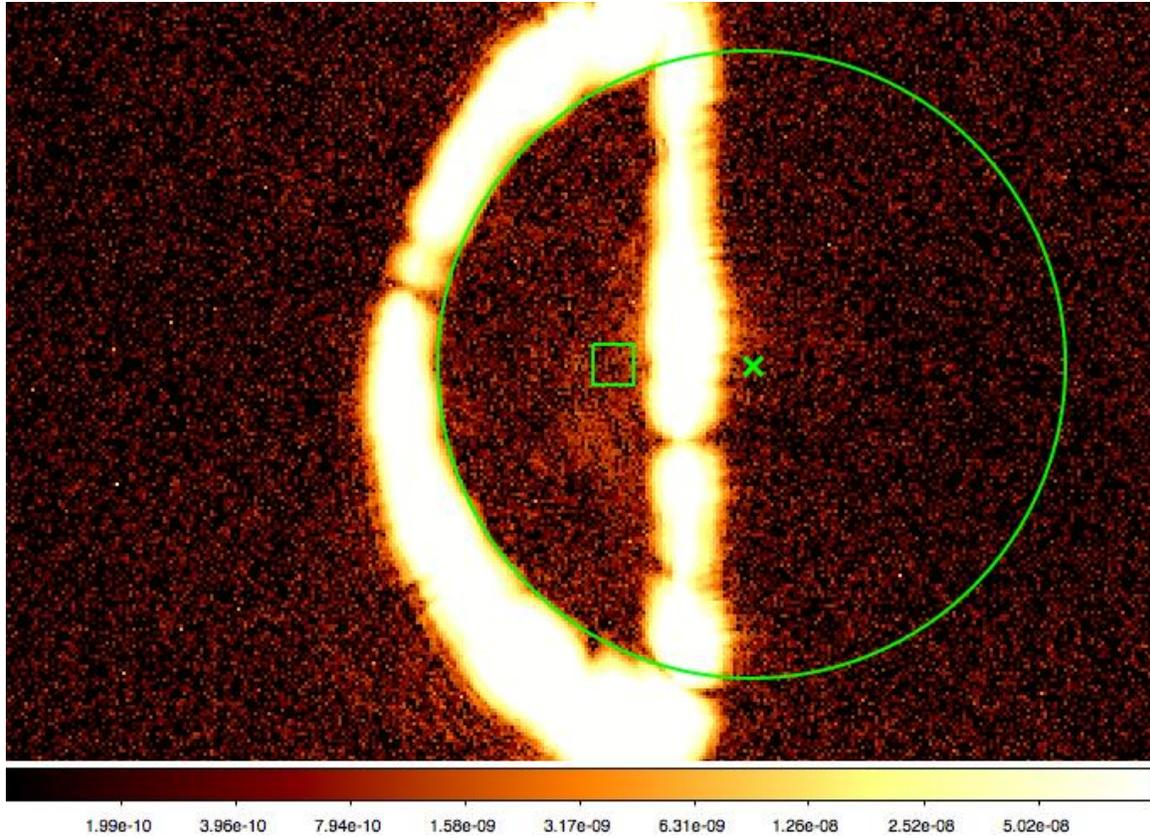
**Figure 8c.** An overlay of an  $8 \lambda/D$  circle, a  $3-4 \lambda/D$  square, and a cross marking the star location on the final dark hole image in our first milestone run.
