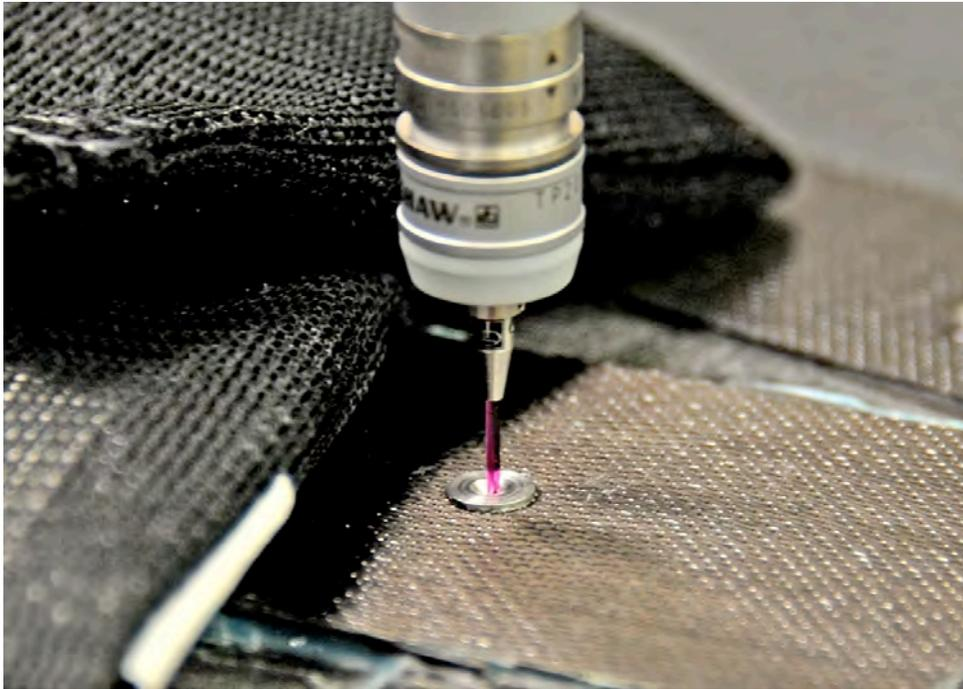
FIGURE 18. Cylindrical probe measuring inside the button at Allied. The edge of the cylindrical probe was also used to measure the edge location.
