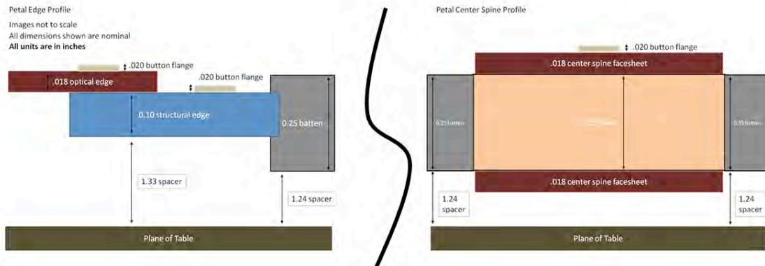
FIGURE 17. Petal assembly dimensions as positioned on the table at Allied.
