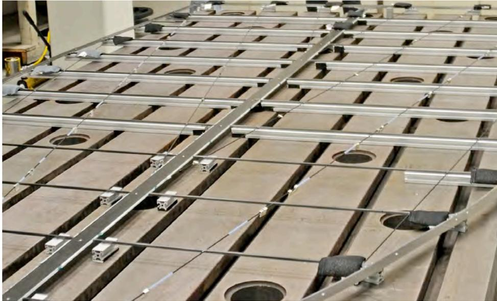
FIGURE 16. Setup of the petal on the tables at Allied. The black and grey bags are bearing-filled bags that load the petal to maintain contact with the extrusion pieces.
