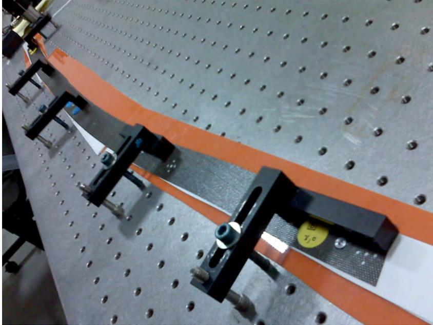
FIGURE 10. Setup of an optical edge for measurement with the FARO arm. Additional weights (not present) were also placed between the fixed clamps. The orange pieces are the low-friction surface and the white pieces are the height shims for the edge.
