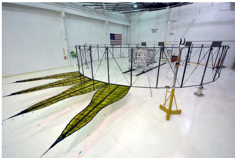
FIGURE 10. The fully deployed truss with attached petals.
