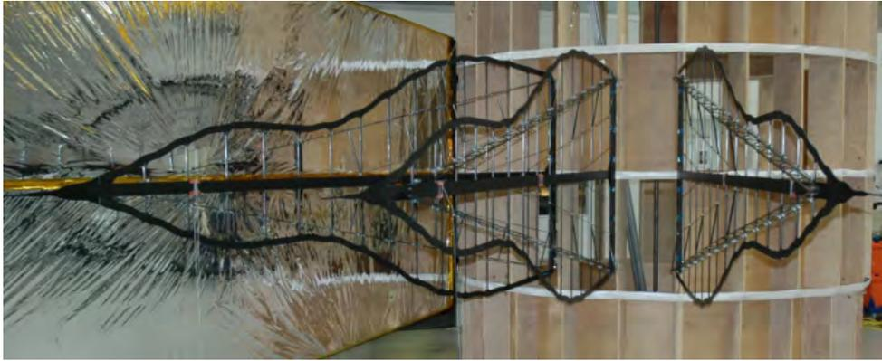
FIGURE 4. As-Built Petals on Mock Hub
