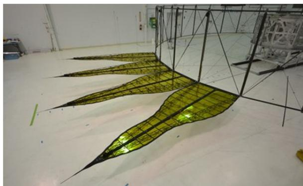
**Figure ES-5.** Deployment demonstration of a partial starshade prototype from 2013 at Northrop Grumman Corporation facilities.
