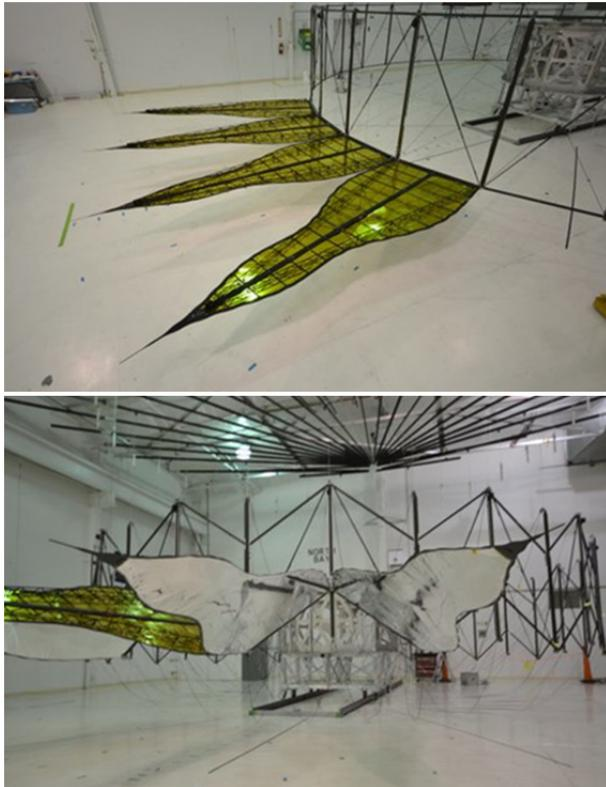
**Figure 6.2-4.** Deployed position tolerance demonstration. Petal root positions are measured after each of 20 deployments.
