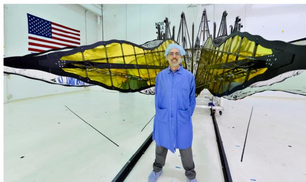
Figure 1.2-3. Starshade stowage and deployment test with four petals. JPL/Princeton/NGC. See also Figure 6.2-3.
