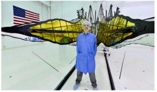
**Figure 1.2-3.** Starshade stowage and deployment test with four petals. JPL/Princeton/NGC. See also Figure 6.2-3.
