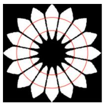
**Figure 6.3-4.** Starshade test article supported by a diffraction controlling outer ring. Red circles indicate the inner and outer working angles.
