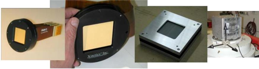
Figure 2. The development of the monolithic PMN deformable mirrors. From left to right: a  $32 \times 32$  mm array (1024 actuators), of the type used for all HCIT demonstrations to date; a  $64 \times 64$  mm array (4096 actuators) first installed on HCIT in 2009; a  $48 \times 48$  mm array (2304 actuators) to be used to demonstrate TRL6 flight-readiness; and the  $48 \times 48$  array on the JPL shake table.
