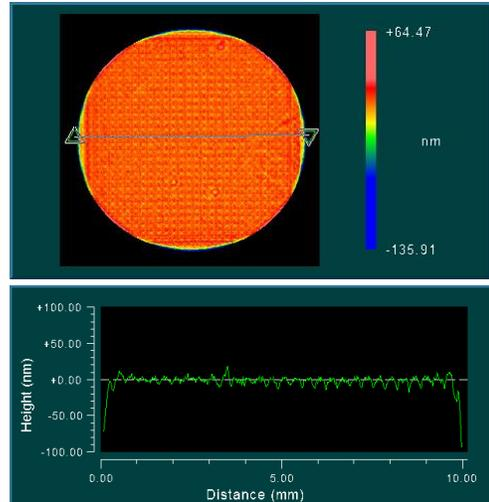
Figure 1: Interferometric surface map of a BMC CDM mirror. Shows surface error of  $R_q = 4.7\text{nm RMS}$
