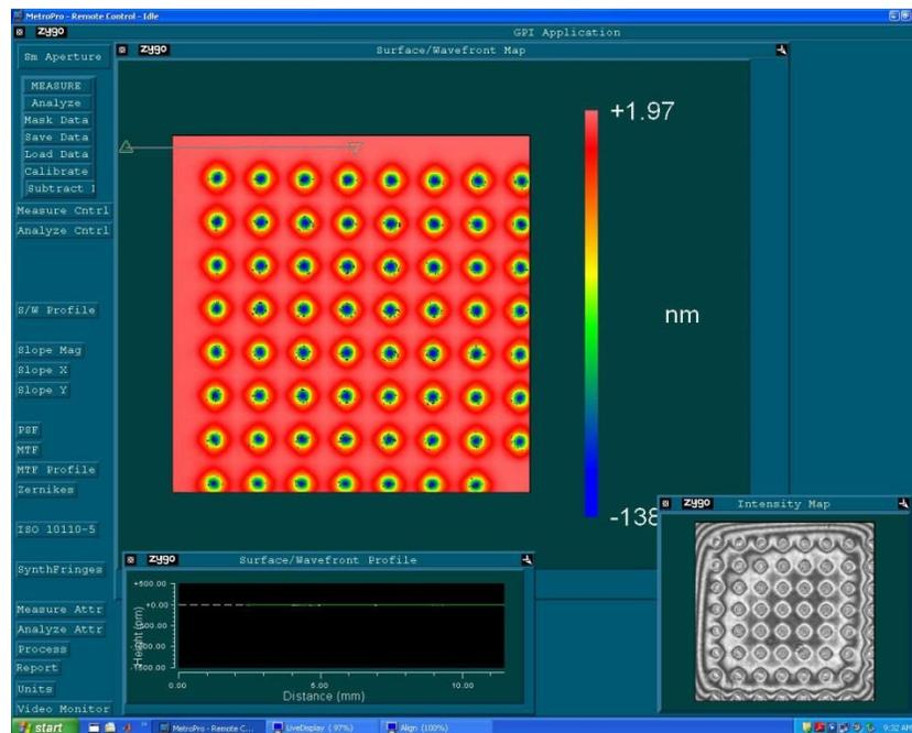
Figure 2: Surface measurement of Kilo-DM with a voltage applied to 64 actuators.
