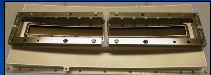
HST-COS far-ultraviolet detector showing the two abutting microchannel plate detector segments (each 85 x 10 mm) curved to the focal plane of the spectrograph.
