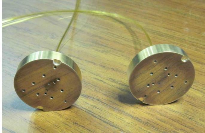
Figure 27 37-fiber Coherent Array
