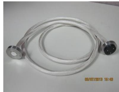
Figure 25 Commercial single mode fiber array (331 fibers)
