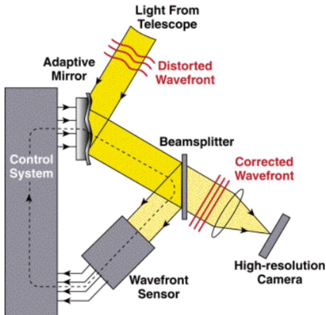
The wavefront actuation is done using a Deformable Mirror.
