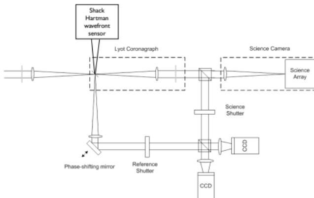
The light after the coronagraph is interfered with some of the light rejected by the coronagraph. The wavefront is retrieved using phase shifting interferometry.
