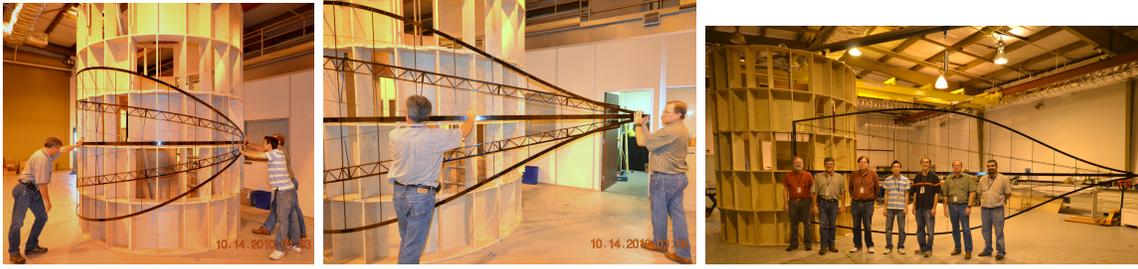
FIGURE 12. Three images of an engineering model petal before, during, and after deployment from a test fixture.
