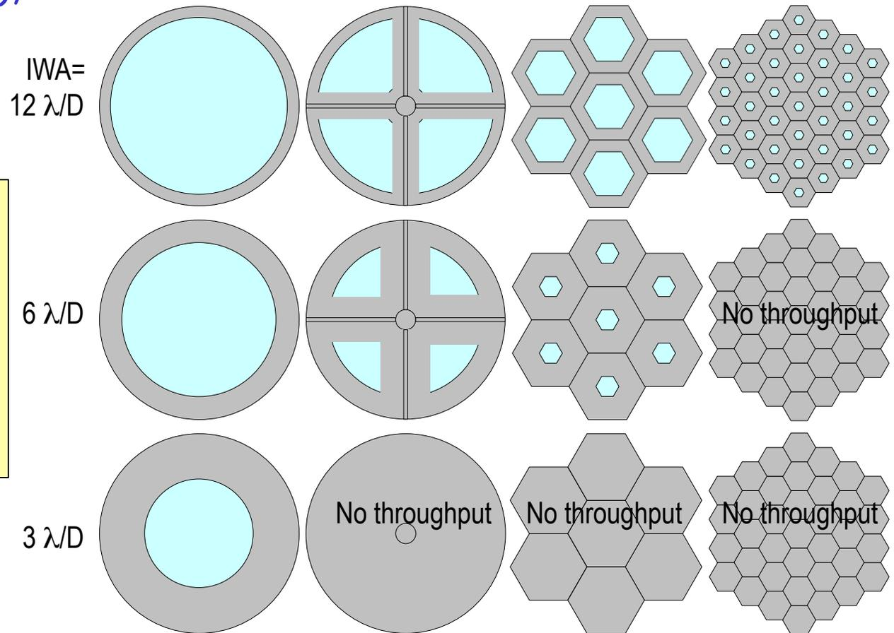
For Lyot coronagraph, as for most (not all) kinds of internal coronagraph, a monolithic unobscured aperture is ~required: the only practical option
