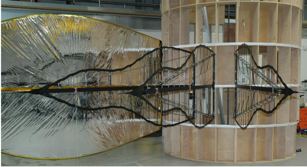
FIGURE 9. Three petals mounted on hub mockup for preliminary deployment testing.
