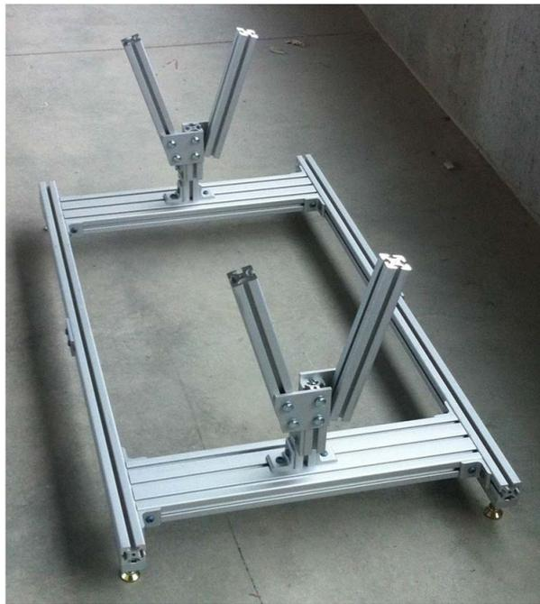
FIGURE 23. Prototype model for the tube support saddles.
