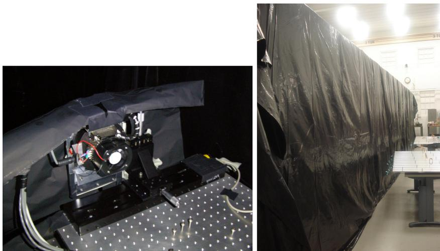
FIGURE 3. *Left:* The occulter camera with baffling. *Right:* Photo of the occulter experiment enclosure in the Gas Dynamics Lab at the Princeton Forrestal Campus.
