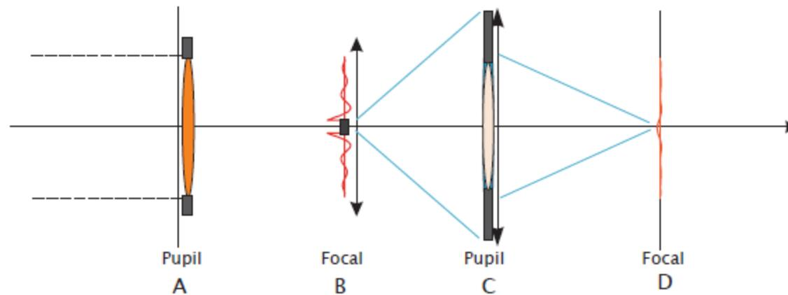
Fig. 1. Illustration of the four coronagraphic planes: the pupil corresponds to Plane A (possibly apodized). A focal mask (hard-edged, or phase mask) is placed in the focal plane B, and a Lyot stop (possibly undersized) in plane C.
