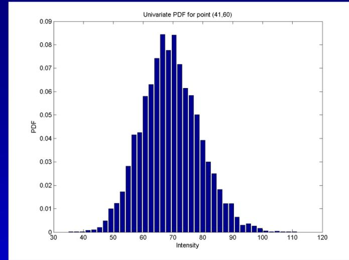
Univariate PDFs for irradiance at two different points in the focal plane
