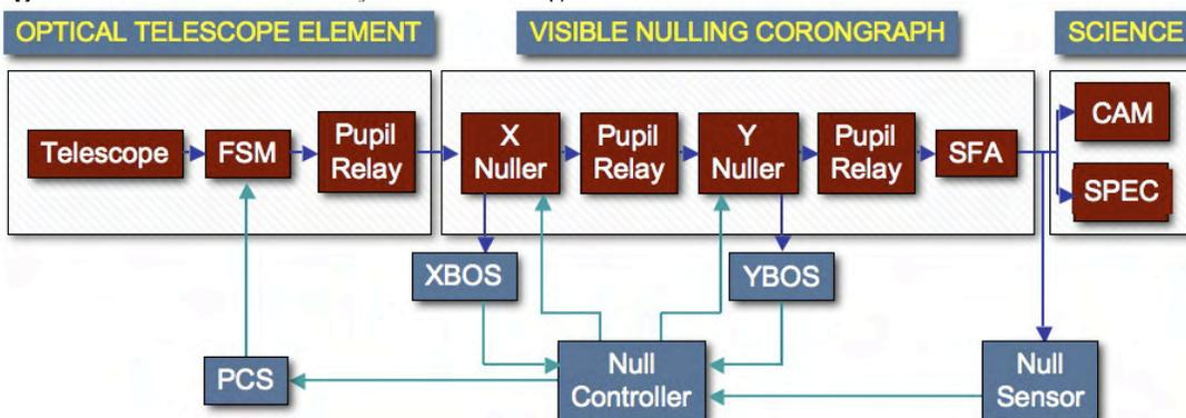
The OTE is an unobscured two-mirror cassegrain telescope with metering truss, support structure, pupil relay and fine steering mirror (FSM); the pupil relay and FSM physically reside within the VNC enclosure to insure stability but are considered as part of the OTE. The VNC contains fore optics which relays the OTE entrance pupil onto the fine steering mirror (FSM) and a pupil relay to relay the pupil at the into the VNC. The VNC performs starlight suppression to
