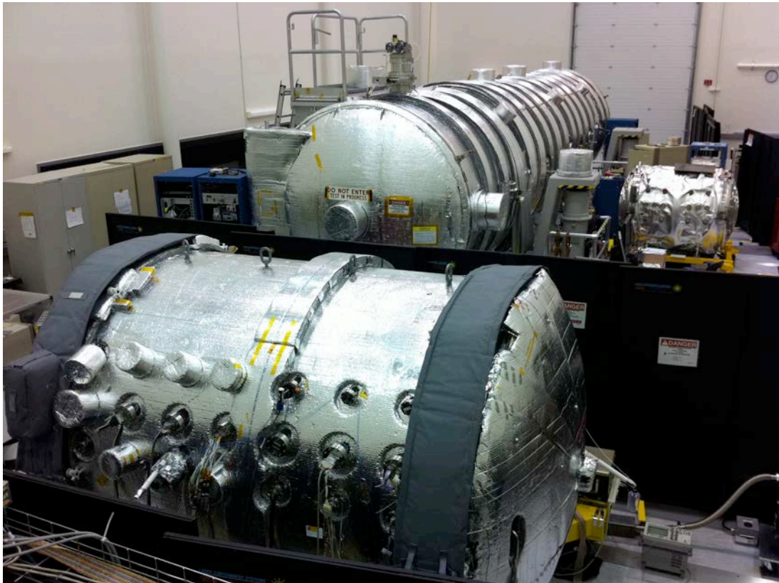
Fig. A.3. The Exoplanet Exploration Program facilities at the Jet Propulsion Laboratory. The High Contrast Imaging Testbed (HCIT-1) is in the foreground. It currently houses experiments that use hybrid Lyot masks and vector vortex masks. The HCIT-2 facility is the large tank in the top center. It currently supports experiments in Phase-Induced Amplitude Apodization (PIAA). The APEP facility, which houses a visible nulling testbed is the smaller tank seen in the upper right of the photo. These facilities are located in the highbay of Building 318.
