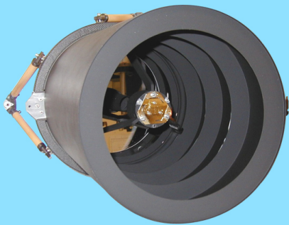
Long Range Reconnaissance Imager (LORRI), Panchromatic Visible Imager, Mass 9.03 kg, Power 4.6 W
