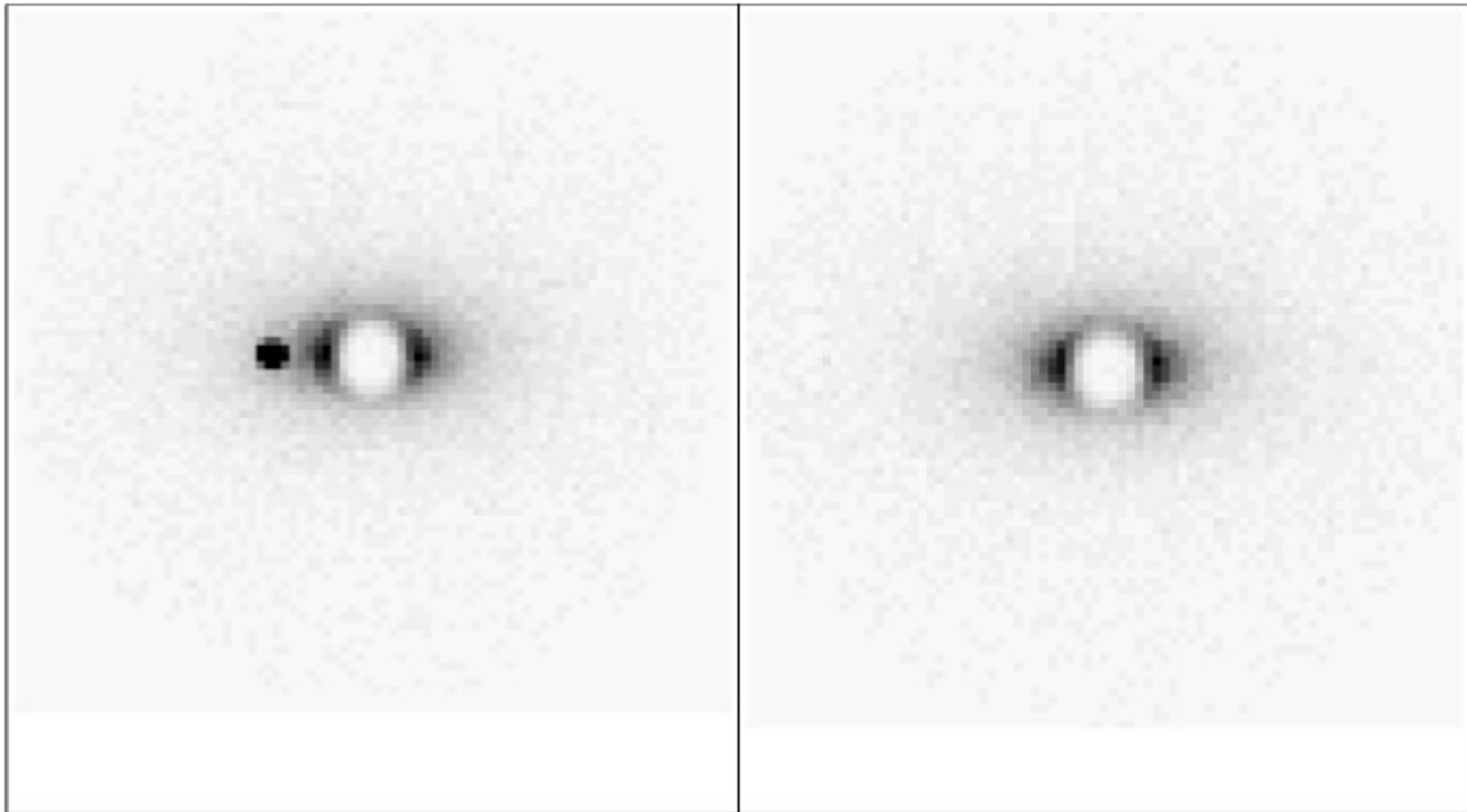
Figure 7-4: Sun at 10 pc with a circumstellar disk and Jupiter (left) and with Earth (right), each 86,400 sec (10 days) integration time. The 10 zodi disk has inclination i = 59 degrees in each image. Jupiter is clearly visible at high signal-to-noise because it is far outside the IWA where the disk surface brightness is low. The Earth has disappeared within the IWA and is drowned by the disk flux.
