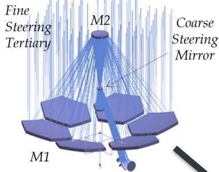
**3 Mirror Anastigmat Telescope (1.45 m aperture)**
