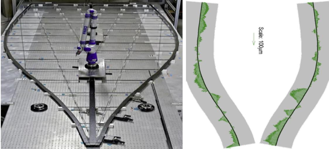
**Figure 23:** Left: prototype petal from TDEM-9. Right: measured errors from nominal shape (green) and bounding envelope meeting suppression requirements (grey).
