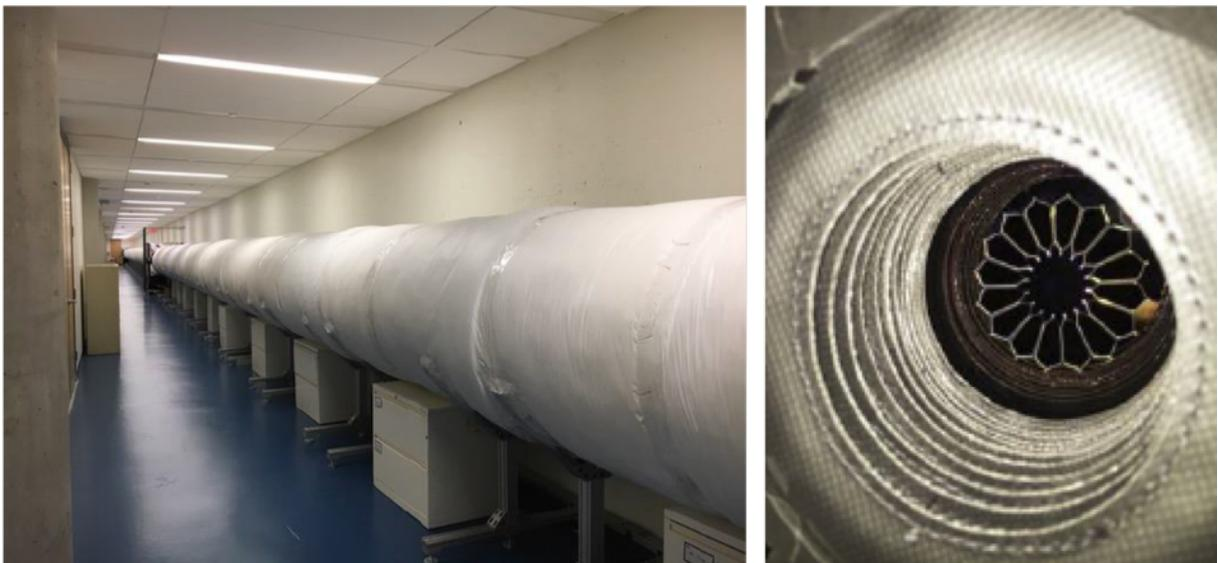
**Figure 5:** Left: The Princeton Frick testbed. Right: a starshade mask as mounted in the testbed.
