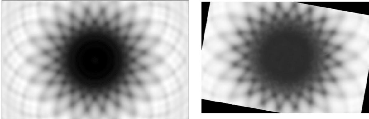
**Figure 15:** Left, starshade shadow in sensing band predicted by optical model. Right, shadow measured in SLATE.
