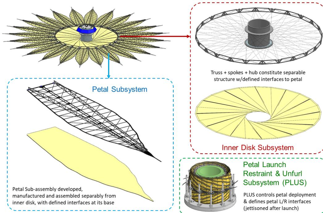
**Figure 16:** Major subsystems of the mechanical architecture.
