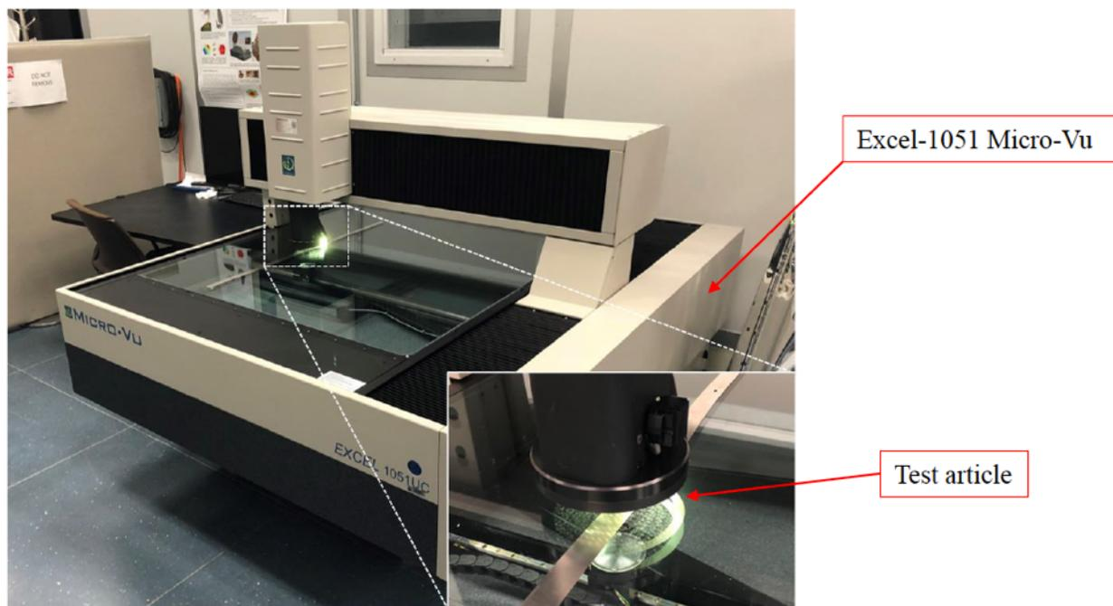
**Figure 24:** Excel-1051 Micro-Vu measurement system.
