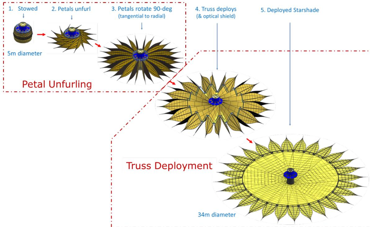
**Figure 17:** Deployment sequence of S5 starshade.
