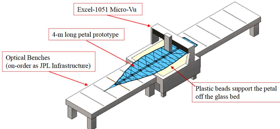
**Figure 25:** Layout of shape metrology for half-scale petal article (test B3).
