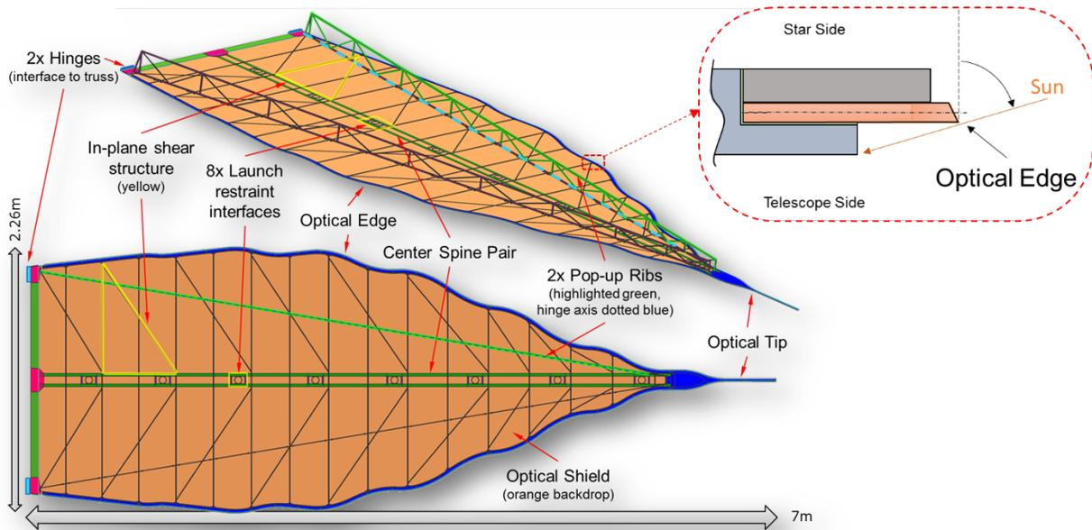
**Figure 19:** Detail of starshade petal, including cross section of optical edge.
