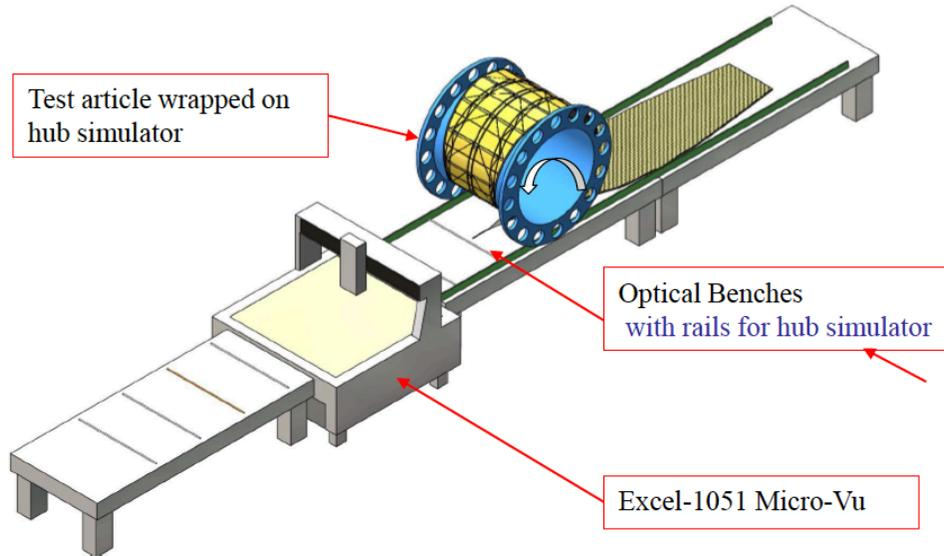
**Figure 26:** Layout of petal furling test B2.
