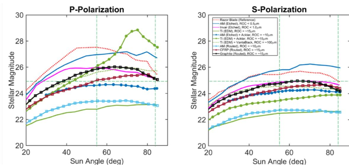
Figure 8: Measured solar scatter, referenced to magnitude at telescope, for candidate edge materials tested. The vertical dashed lines show the allowable limits of incident Sun angles in the Starshade Rendezvous mission. The horizontal dashed line shows the minimum acceptable magnitude of scatter.
