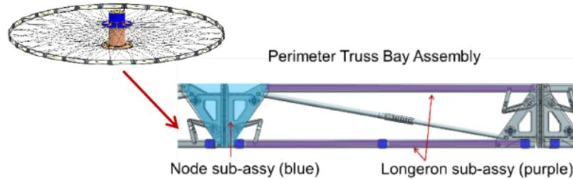
**Figure 22:** Truss bay assembly, showing its location within inner disk and locations of longeron and node subassemblies.
