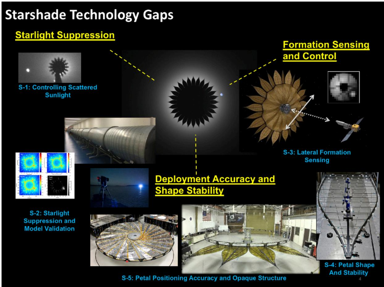
Figure 1: Starshade technologies and technology gaps.
