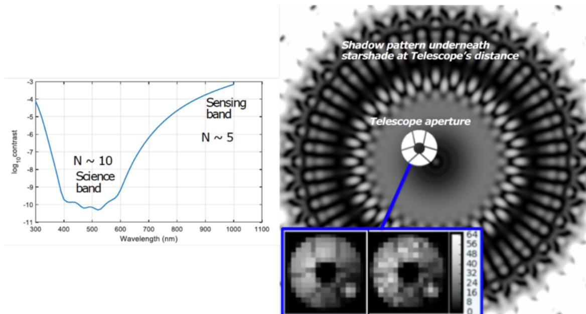
**Figure 13:** Left, suppression vs. wavelength of starshade, showing both science and sensing regions. Right, modeled starshade suppression pattern in sensing band with WFIRST aperture shown for scale. Inset, predicted lateral sensing image at WFIRST pupil plane, with and without simulated noise.
