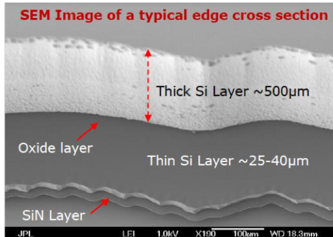
**Figure 6:** Cross section of typical mask edge.
