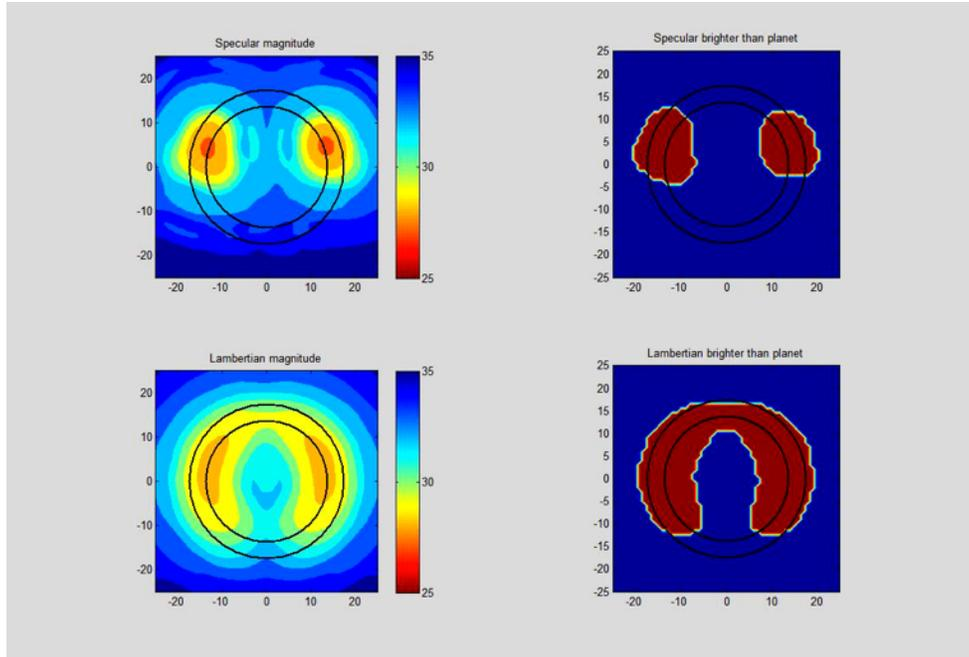
Figure 7: Solar scatter from starshade as seen by WFIRST.
