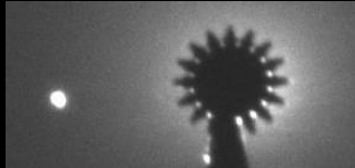
Suppressing scattered light off petal edges from off-axis Sunlight (S-2)
