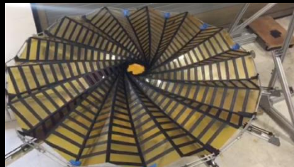
Positioning the petals to high accuracy, blocking on-axis starlight, maintaining overall shape on a highly stable structure (S-5)
